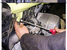
To raise the tank is a extremely easy operation. He is sufficient to unscrew the only screw to present brugola on the skillful, accessible side being removed the lateral in fixed black plastic to pressure. After to have unscrewed the bolt, the tank is free to slide to behind and can be raised without difficulty.
