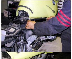
The installation of eprom the TRITON previews the substitution of chip in the central unit the Bosch Motronic BUT 2,2, situated under the tank of the fuel.
