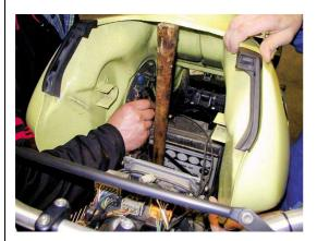
In order to approach the telephone exchange, the tank of the fuel can simply be raised or taken apart entire. In this last case, but, it is necessary to d3connecter the wiring electrical worker of the pump of the fuel and the small tubes of flow of the fuel, being had the shrewdness to obstruct of the escape.
