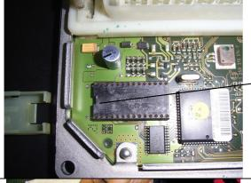
You take in hand eprom the Triton and identify the back of insertion, given from the notch on the high part of the eprom and from the support in black plastic where heel is present one and insert delicately. The two heels will be therefore one over to the other. Attention: the corrected insertion of the Eprom inside avoids the loss total of the data of the same one damaging itself.
