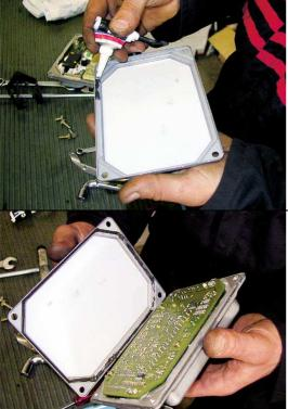
Before close the central unit be advisable restore the seal a of the semishell with of the common silicone.
