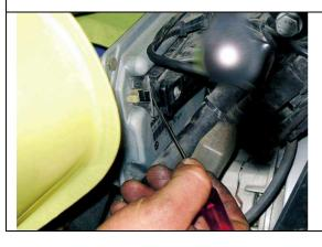
In order to unblock the large connector of the telephone exchange it is necessary to uncouple with a screwdriver the clip of detention in steel situated on the skillful side.
