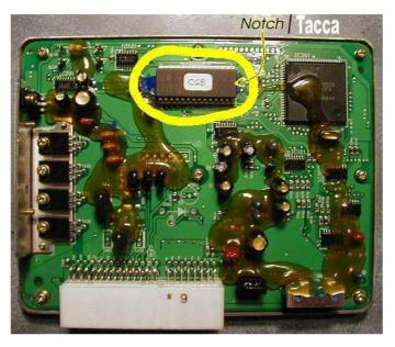
You take in hand eprom the Triton delicately and indentificate the back of insertion, given from the notch on the high part of the eprom and from the design on the green slab and insert.
