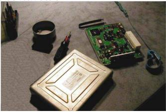
To identify the position of the Eprom originates them and with a screwdriver to flat head. To remove inserting it delicately it between eprom and the card before from a part and then from the other. Therefore you will avoid to fold the piedini of the
